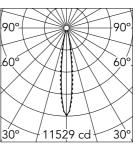
Luminous flux luminaire 1411 lm
