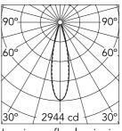
Luminous flux luminaire 685 lm
