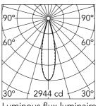
Luminous flux luminaire 685 lm
