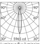
Luminous flux luminaire 730 lm
