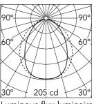
Luminous flux luminaire 448 lm
