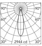
Luminous flux luminaire 685 lm
