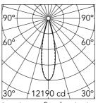
Luminous flux luminaire 2836 lm
