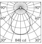
Luminous flux luminaire 1856 lm
