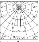
Luminous flux luminaire 2754 lm
