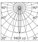
Luminous flux luminaire 2662 lm
