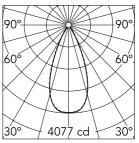
Luminous flux luminaire 2728 lm
