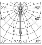
Luminous flux luminaire 2754 lm
