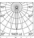
Luminous flux luminaire 2662 lm
