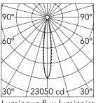
Luminous flux luminaire 2821 lm
