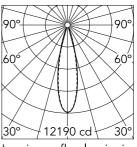
Luminous flux luminaire 2836 lm
