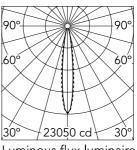
Luminous flux luminaire 2821 lm
