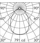
Luminous flux luminaire 1732 lm
