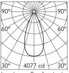
Luminous flux luminaire 2728 lm
