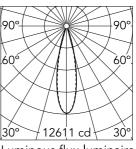
Luminous flux luminaire 2934 lm
