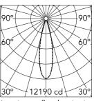
Luminous flux luminaire 2836 lm
