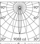
Luminous flux luminaire 2571 lm
