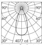
Luminous flux luminaire 2728 lm
