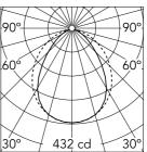
Luminous flux luminaire 930 lm
