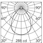
Luminous flux luminaire 620 lm
