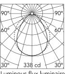
Luminous flux luminaire 728 lm
