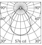
Luminous flux luminaire 1240 lm
