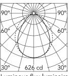
Luminous flux luminaire 1348 lm
