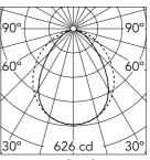
Luminous flux luminaire 1348 lm
