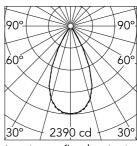
Luminous flux luminaire 1672 lm
