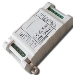
1-10V PWM control interface 48Vdc 120W IP20. Power supply not included
