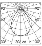
Luminous flux luminaire 414 lm
