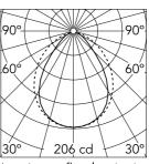
Luminous flux luminaire 414 lm
