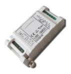
1-10V PWM control interface 24Vdc 120W IP20. Power supply not included F990B14A000
