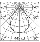
Luminous flux luminaire 894 lm
