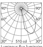
Luminous flux luminaire 656 lm
