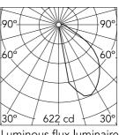
Luminous flux luminaire 800 lm
