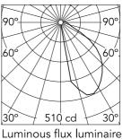
Luminous flux luminaire 656 lm
