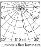
Luminous flux luminaire 656 lm
