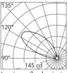
Luminous flux luminaire 472 lm
