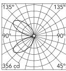
Luminous flux luminaire 1020 lm
