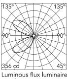
46° Beam Angle DIR: h(m) E(Ix) D(m) 356 2.69 1 5.39 2 89 3 40 8.08 4 22 10.77 5 14 13.47
