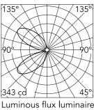
46° Beam Angle DIR: h(m) E(Ix) D(m) 343 2.69 1 5.39 2 86 3 38 8.08 4 21 10.77 5 14 13.47
