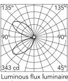
46° Beam Angle DIR: h(m) E(Ix) D(m) 343 2.69 1 2 5.39 86 3 38 8.08 4 21 10.77 5 14 13.47
