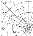
Luminous flux luminaire 472 lm
