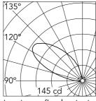
Luminous flux luminaire 472 lm
