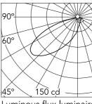
46° Beam Angle: h(m) E(Ix) D(m) 150 2.69 1 5.39 2 38 3 17 8.08 4 9 10.77 5 6 13.46
