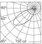
Luminous flux luminaire 491 lm
