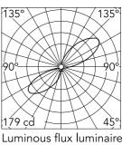
45° Beam Angle DIR: h(m) E(Ix) D(m) 179 2.68 1 2 5.37 45 3 20 8.05 4 11 10.73 5 7 13.42
