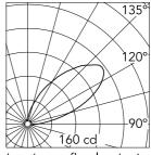
Luminous flux luminaire 503 lm
