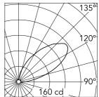
Luminous flux luminaire 503 lm
